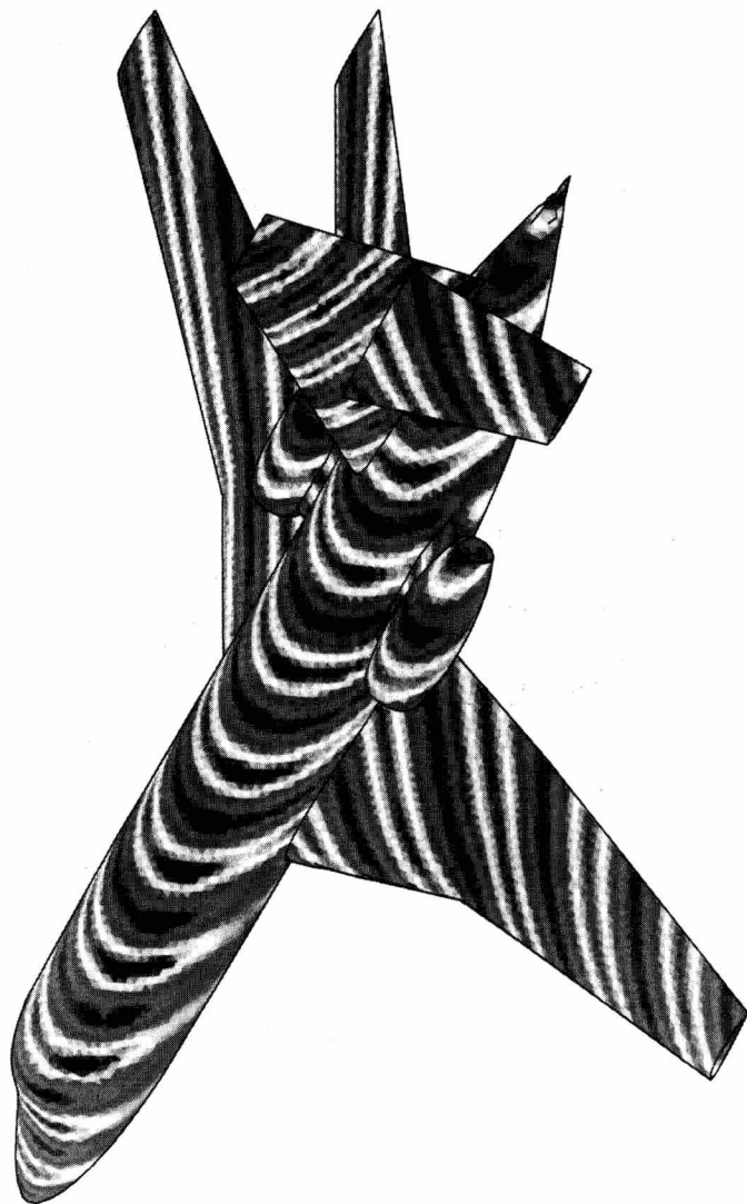
Plate 4 Scattering of a plane electromagnetic wave by a perfectly conducting aircraft
