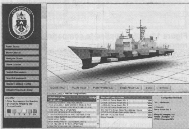
Figure 9: Cumulative view of affected compartments for an overhaul or availability
