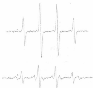
FIGURE: A) typical \text{HO}\cdot signal from \text{O}_3 and phosphate/caffeic acid, B) same as A but with 0.6 M sorbitol, note side bands.
