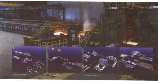
Integrated CSP casting/rolling plant. Coupling-together of process stages increases the economy and shortens the production process.
