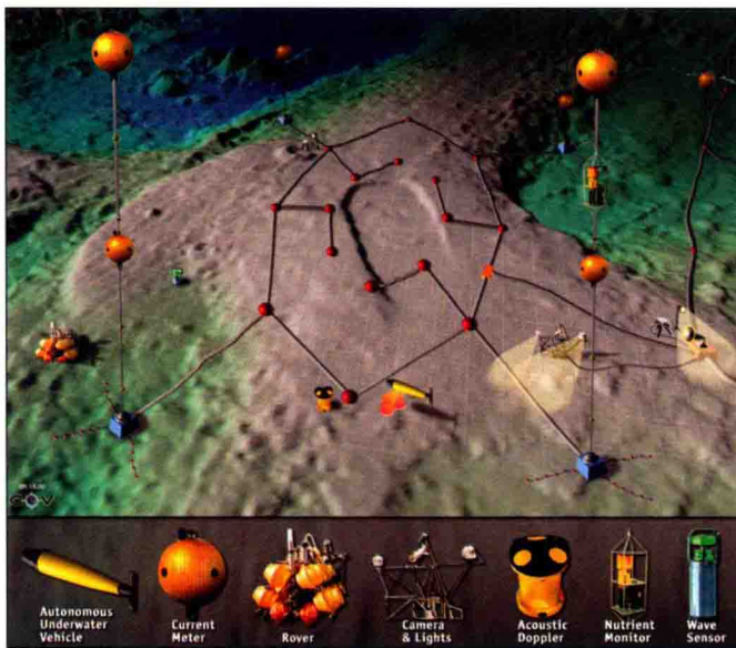
Figure 1.1 The North-East Pacific Timeseries Undersea Networked Experiments (NEPTUNE) ocean observatory envisions a hypothetical network of oceanographic instruments and vehicles to be deployed on Axial Volcano in the northeast Pacific Ocean. It is based on the existing NOAA New Millennium Observatory (NeMO) on Axial. This image also shows the many and varied sources of data that may be available from one major study site for marine GIS maps and analyses.
