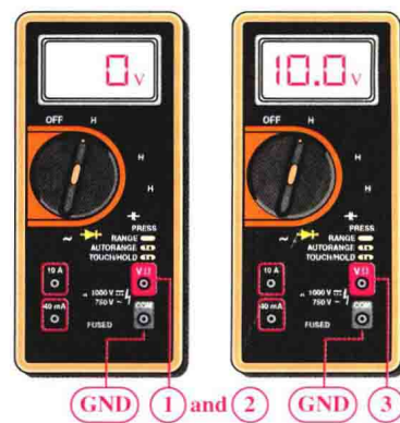
(c) The voltage is found at point ③, indicating that one of the two used protoboard contacts in that row is bad.
