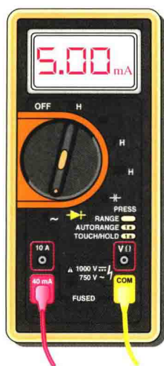
(a) Meter with yellow lead going to protoboard and red lead going to the positive terminal of the 25 V power supply.
