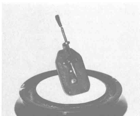
Fig. 1-1. Antony van Leeuwenhoek's microscope. A replica of one of the first microscopes made by Leeuwenhoek about 1673. A single little lens is in the peephole in the flat plate. The object to be viewed is placed on the spike and adjusted with screws. The microscope is held close to the eye for viewing. It provides magnifications of about 200\times to 300\times . (Courtesy of Armed Forces Institute of Pathology, Washington, D.C.)
