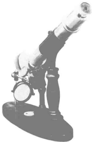
Fig. 1-3. The Holmes microscope. A compound microscope devised by Oliver Wendell Holmes in 1873. A magnification of approximately 400\times could be obtained. (Courtesy of Armed Forces Institute of Pathology, Washington, D.C.)
