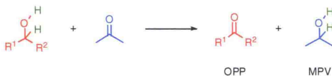
Fig. 1.3 Oppenauer oxidation using acetone as the sacrificial agent. OPP = Oppenauer oxidation (product). MPV = Meerwein-Ponndorf-Verley (product). Two hydrogen atoms are extruded from the red-colored alcohol and given to the blue-colored carbonyl substrate (acetone in this example). R-substituents constitute alkyl and aryl substituents
