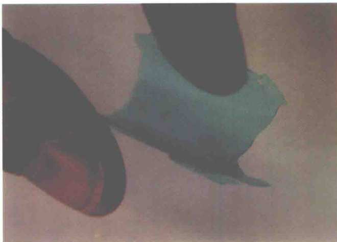
A thin, clear blue film of chitosan/Y124 superconductor precursor.
