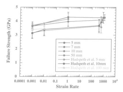
Fig. 1.1 Tensile strength as a function of strain rate
