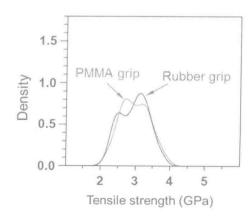
Fig. 2.1 Kernel density plot for the fiber strengths obtained by PMMA and rubber grips
