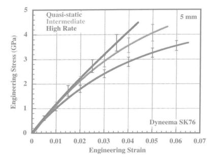
failure strength of Dyneema does not depend on the gage length of the fiber since no change in strength was observed at shorter gage lengths. Future work should include shorter gage lengths to further probe this observation. The results of this study show higher failure strengths compared to the study by Hudspeth et al. [5] on Dyneema SK76, but compare well with published data by Dyneema [14] and a study by Russell et al. on SK76 fibers and yarns [3].
