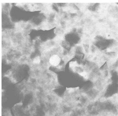
Figure 3. Montmorillonite, (\text{Mg,Ca})\text{O} \cdot \text{Al}_2\text{O}_3 \cdot 5\text{SiO}_2 \cdot n\text{H}_2\text{O} —Microcrystalline aggregates of fine scalelike crystals. Mono-
