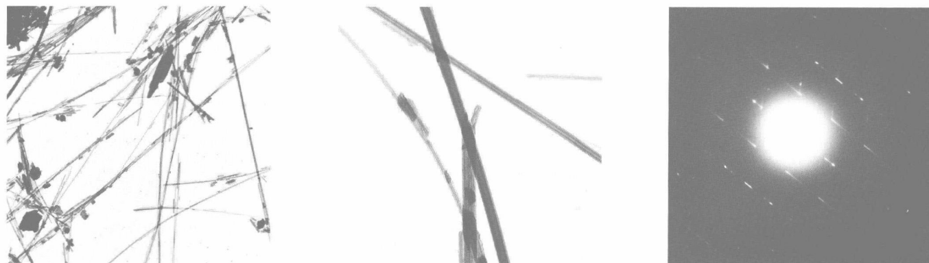
Figure 8. Chrysotile, \text{Mg}_3\text{Si}_2\text{O}_5(\text{OH})_4 (cf. 122)—The most common asbestos forms hollow tubes like halloysite, but the fine chrysotile fibers are more uniform in size and show, of
