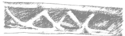
Figure 2 Bow and lattice structure of the currach, an Irish workboat. Stresses on the hull are evenly distributed through the longitudinal stringers, which are held together by steam-bent oak ribs.
