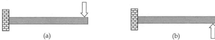
Fig. 1.4 Bending takes place at one end only in in-plane flexural (cantilever) action. One end of a cantilever is fixed against all movements. (a) Hogging cantilever action (b) Sagging cantilever action.
