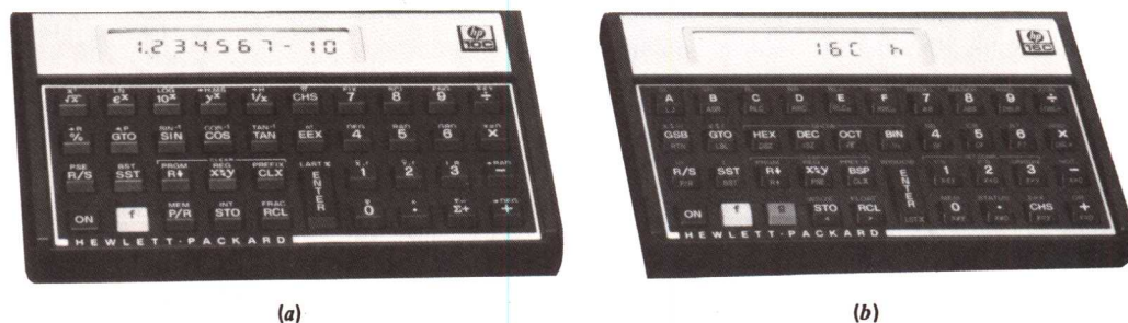
Fig. S-6 Two examples of programmable electronic calculators. Width is about 6 in. (a) Scientific type with exponents, logarithms, and trigonometric functions for sine (SIN), cosine (COS), and tangent (TAN) of angles. (b) Type for digital electronics and computer science. Functions included are for decimal (DEC), hexadecimal (HEX), octal (OCT), or binary (BIN) numbers. (Hewlett-Packard)
