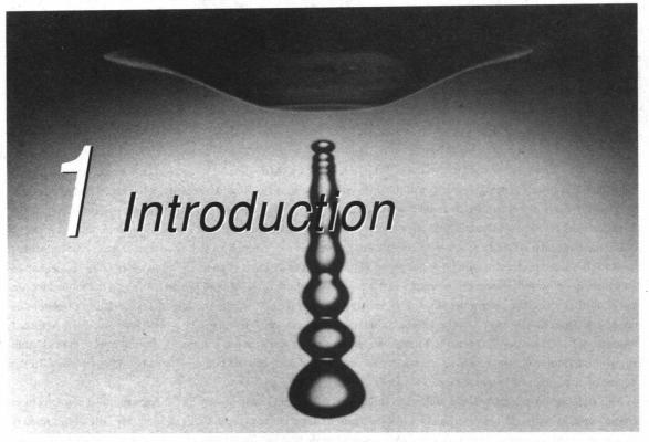
CHAPTER OPENING PHOTO: The breakup of a fluid jet into drops is a function of fluid properties such as density, viscosity, and surface tension. [Reprinted with permission from American Institute of Physics (Ref. 6) and the American Association for the Advancement of Science (Ref. 7).]
