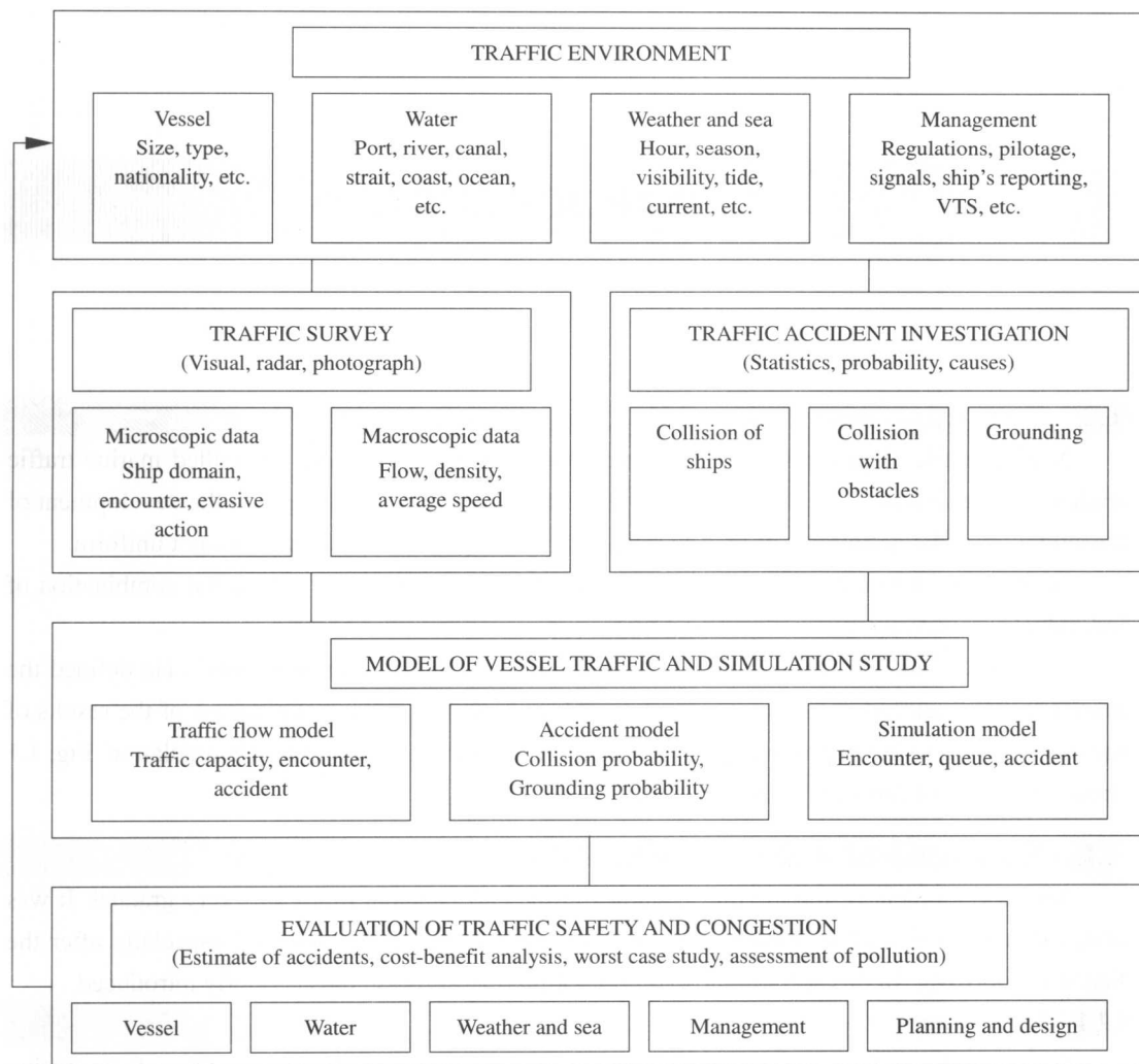
Fig. 1.1 The scope of marine traffic engineering
