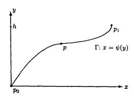
The direct problem is to determine the time T in which the element moves from  $p_1$  to  $p_0$  when the curve  $\Gamma$  is given. In the inverse problem, one measures the time T = T(h) for several values of h and tries to determine the curve  $\Gamma$ . Let the curve be parametrized by  $x = \psi(y)$ . Let p have the coordinates  $(\psi(y), y)$ .
