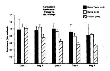
Fig. 1: Change in resistance with time for bone specimens stored in different environment.
