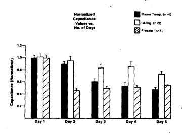
Fig. 2: Change in capacitance with time for bone specimens stored in different environment.
