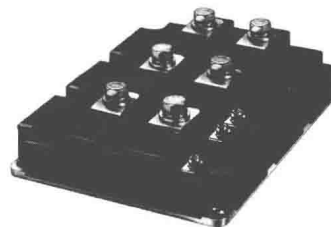
Figure 1.6 High power IGBT (Insulated Gate Bipolar Transistor) as used in a frequency converter
