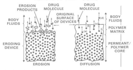
Figure 1.1 Schematic diagram of bioerodable and diffusional systems for drug delivery
