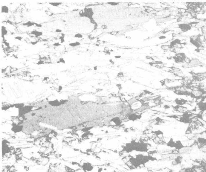
Figure 8: A typical greenschist from Scotland; the gray minerals are biotite and chlorite showing strong preferred orientation. The black crystals are magnetite, and the white areas are albite-quartz. Epidote and calcite are also present (magnification 50 X).
