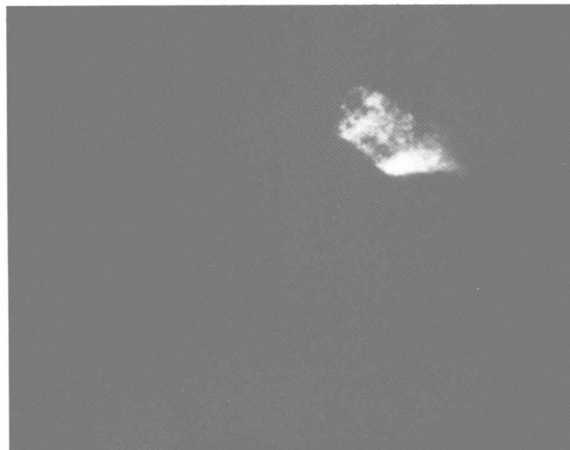
Figure 12. MOLE image of sulfur utilizing 474\text{ cm}^{-1} Raman line for image formation.
