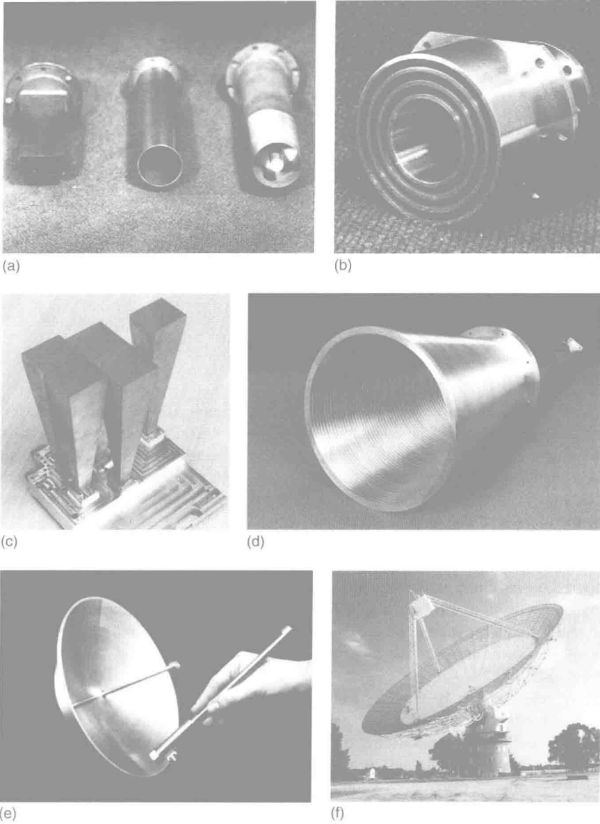
Figure 1.1 Examples of aperture antennas. (a) Open-ended waveguide antennas (right to left) coaxial, circular and rectangular. (b) Circular waveguide (diameter 32.7 mm) with three ring-slots designed for operation at 9 GHz. (c) Feed array of pyramidal horns for 12.25–12.75 GHz. (d) 11–14.5 GHz high-performance circular corrugated feed horn, diameter 273 mm, and flare angle 11.8^\circ . (e) Small paraboloidal reflector and rear waveguide feed designed for a 15 GHz microwave link. (f) 64 m Parkes radio telescope is a front-fed paraboloid ( f/D = 0.408 ). This versatile instrument has been used for frequencies from 30 MHz to >90 GHz. Source: Reproduced with permission from CSIRO (a–f)
