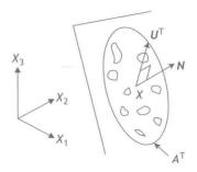
Fig. 1.3 Areal porosity at point *X* in a plane with normal *N*.
