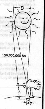
1. Poke a small hole in a piece of card. Perhaps an index card will do, and poke the hole with a sharp pencil or pen. Hold the card in the sunlight and note the circular image that is cast. This is an image of the Sun. Note that its size doesn't depend on the size of the hole in the card, but only on its distance. The image is a circle when cast on a surface perpendicular to the rays-otherwise it's "stretched out" as an ellipse.
