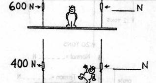
2. When Burl the painter stands in the exact middle of his staging, the left scale reads 600 N. Fill in the reading on the right scale. The total weight of Burl and staging must be
