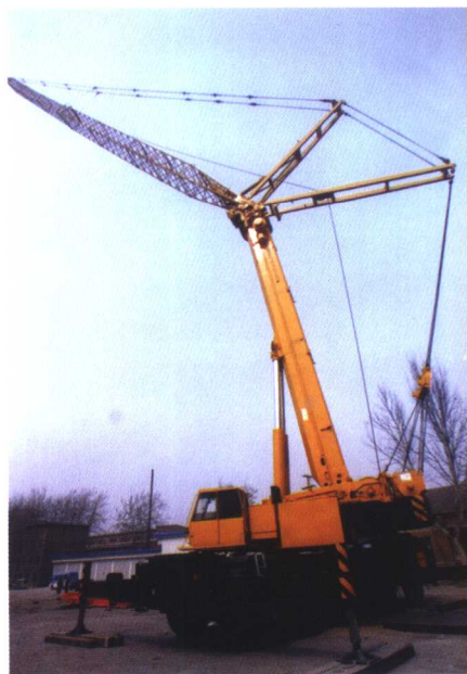
利勃海尔170T吊车 LIEBHERR CRANE
