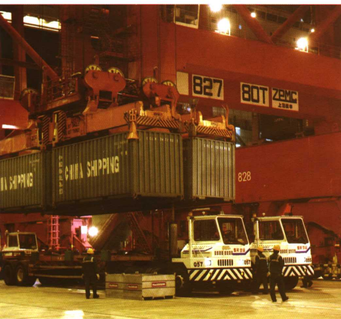
ZPMC 自行研制、拥有自主知识产权的双 40ft 集装箱起重机在上海市洋山港作业 The Twin 40' STS cranes at the Yangshan Port, China, which are developed by ZPMC with independent intellectual property rights
