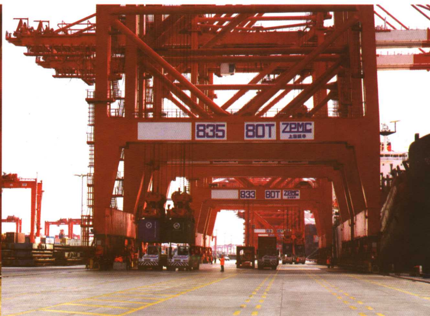
ZPMC 自行研制、拥有自主知识产权的双 40ft 集装箱起重机在上海市洋山港作业 The Twin 40' STS cranes at the Yangshan Port, China, which are developed by ZPMC with independent intellectual property rights
