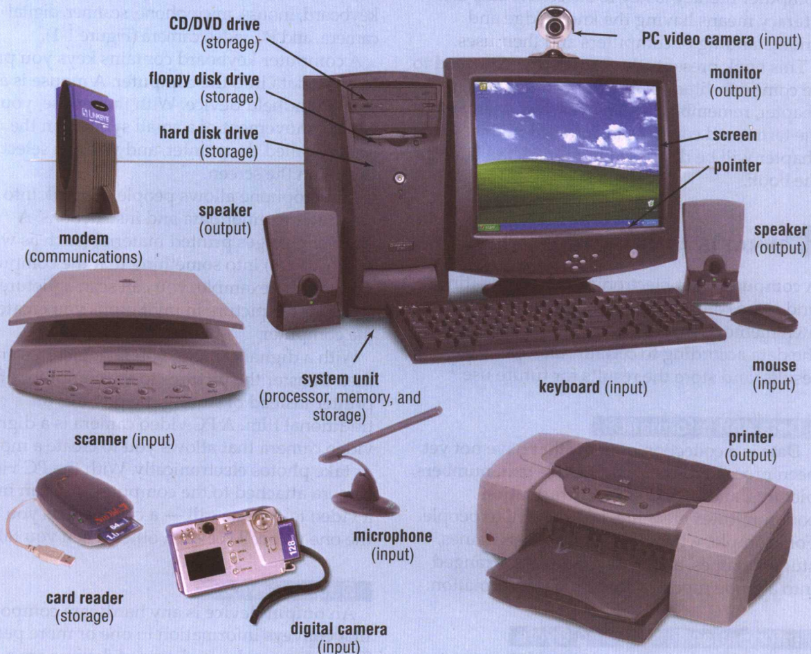
FIGURE 1-1 Common computer hardware components include the keyboard, mouse, microphone, scanner, digital camera, PC camera, printer, monitor, speakers, system unit, disk drives, card reader, and modem.
