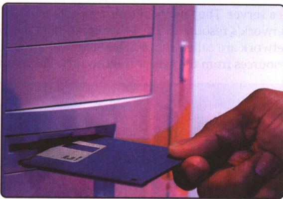
FIGURE 1-2 A floppy disk is inserted in and removed from a floppy disk drive.
