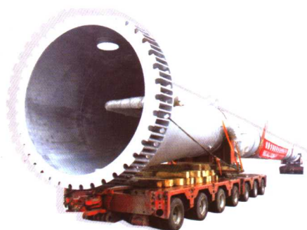
为珠海BP制造的62m钛烟筒 ( \phi 2000, \phi 3600mm, 86t, L=62000mm, 16MnR/Ti; \delta =22+3mm)
