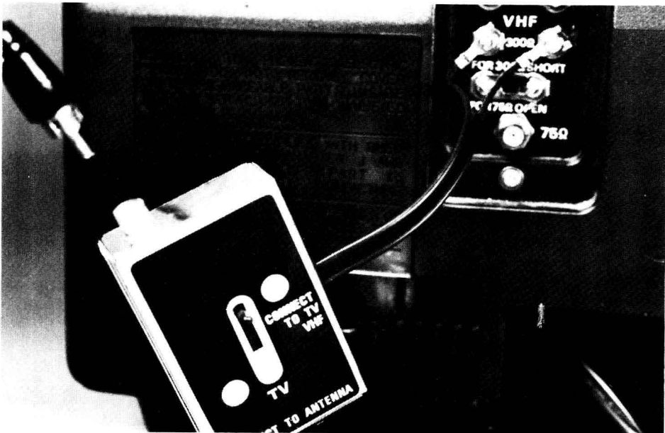
FIGURE 1-4. Television switch box and connections
