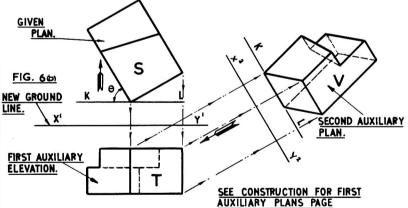
VIEWS SAND T-PEPRESENTING A PLAN AND ELEVATION DRAWN IN THEIR CONVENTIONAL POSITIONS RELATIVE TO THE GROUND LINE X'Y.
