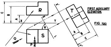
VIEWS RAND S.— STANDARD ELEVATION AND PLAN VIEW\_IN FIRST ANGLE ORTHOGRAPHIC PROJECTION:
