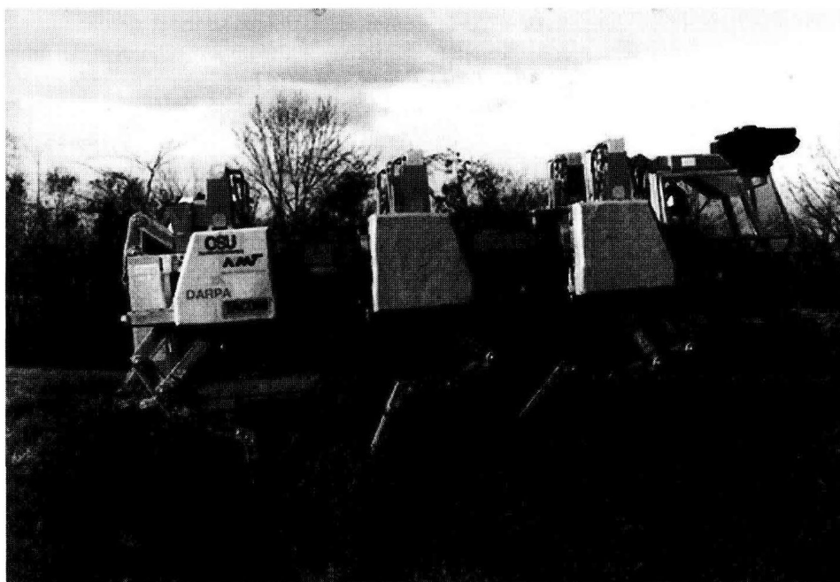
FIGURE 1.1 The Adaptive Suspension Vehicle. Each leg is a planar pantograph mechanism hinged to the body about an axis parallel to the longitudinal axis of the vehicle.
