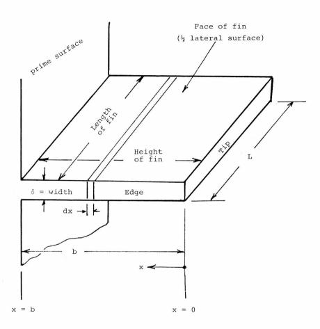
Fig. 1.1. Terminology and coordinate system, longitudinal fin of rectangular profile.
