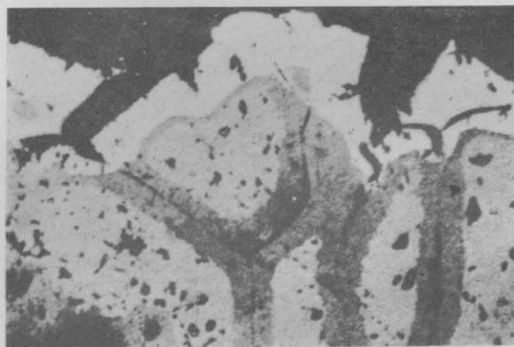
Fig. 5.—Photomicrograph of \text{Fe}_2\text{O}_3 specimen partially reduced in hydrogen at 590^\circ\text{C} ( \times 200 ); white phase iron metal, dark grey phase \text{Fe}_3\text{O}_4 , light grey phase \text{Fe}_2\text{O}_3
