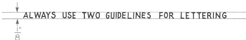
Figure 3-4: Lettering is done between two sharp, thin, light lines called guide lines.
