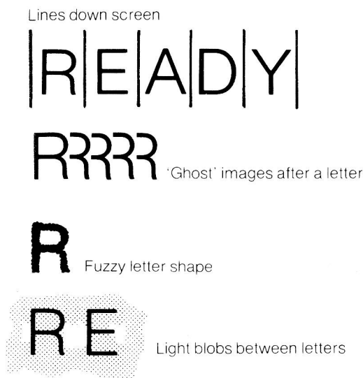
Fig. 1.6. Picture defects caused by faulty tuning.
