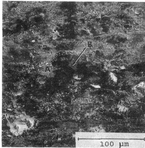
FIG. 6—Wear surface features on alumina pin in the case of pin-on-disk configuration with alumina pin rubbing against tool steel disk.
