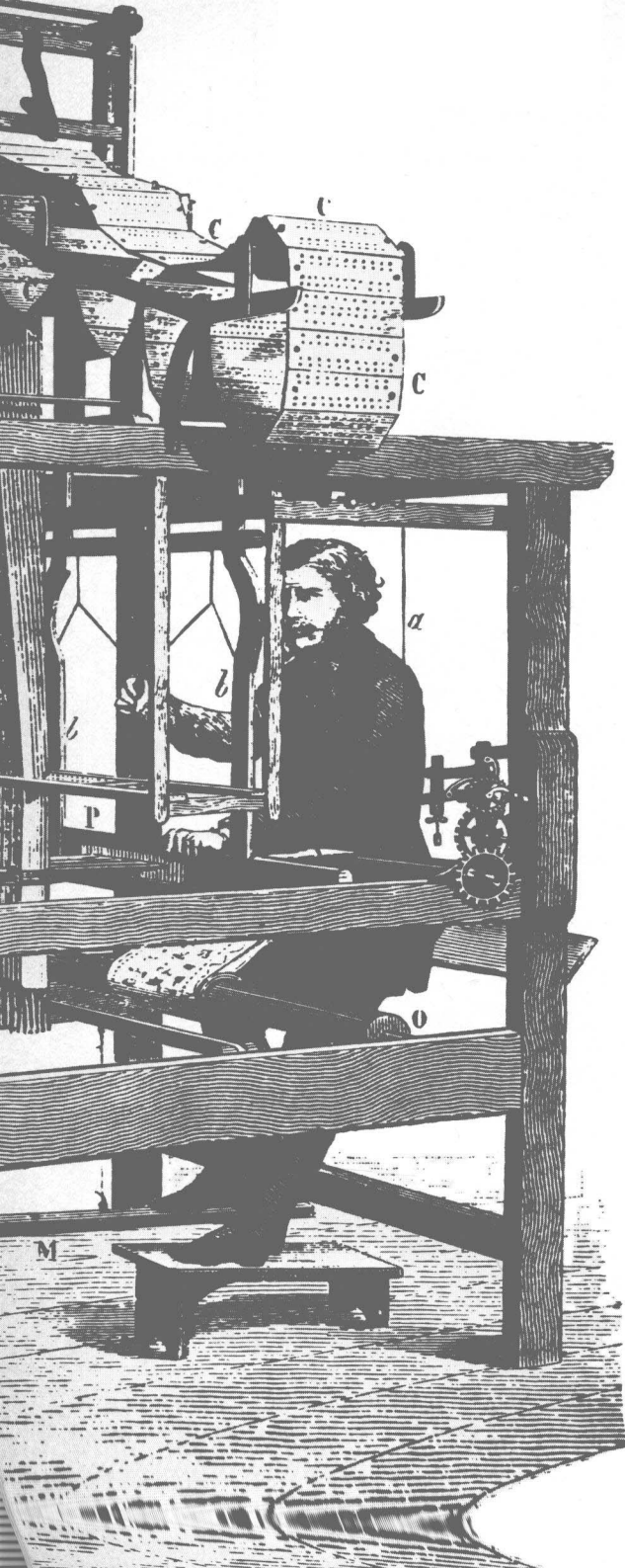
Jacquard loom cards Used to determine the pattern of the weave, this development marked the beginning of punch card accounting and programming.
