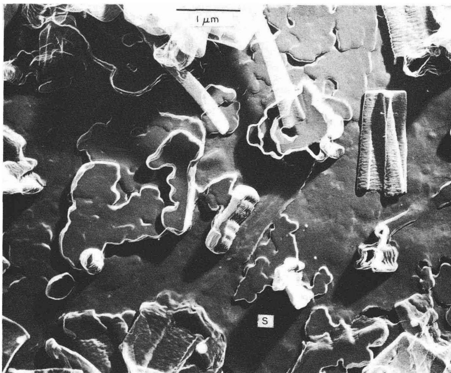
Fig. 2-3 A platinum-shadowed carbon replica of a cabbage ( Brassica oleracea ) leaf surface. (S) is the 'shadow' formed by the exclusion of platinum from the carbon surface.
