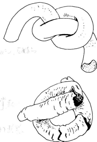
Fig 7. Plastic and short clays are assessed quickly by the tie-a-knot test.
