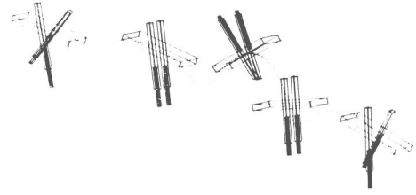
Figure 4: Cartoon of planar biped doing a forward flip. The machine was running from right to left. 1) Approach with normal alternating gait, 2) hurdle step to gain altitude and prepare for double support, 3) the body has accelerated forward to initiate the flip and the legs have shortened to increase pitch rate, 4) landing step reduces pitch and vertical rates, and 5) resume normal alternating gait. The body configurations are from actual data recorded during a flip. The dots indicate the path of the center of mass at 12 ms intervals.
