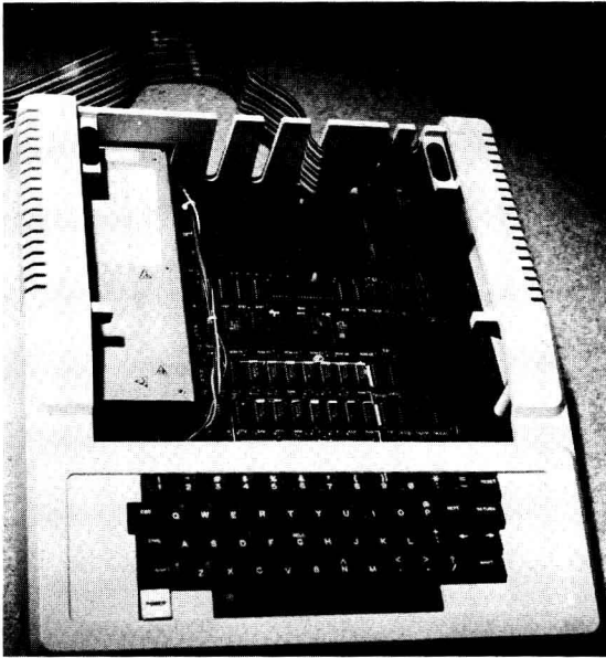
Figure I-2 (a) Apple computer with its cover removed, revealing the Vector Electronics plugboard in slot 7. The ribbon cable connected to the rear of this card provides access to the interfacing signals required to do the experiments. A solderless breadboard is used to build up the various interfacing circuits.
