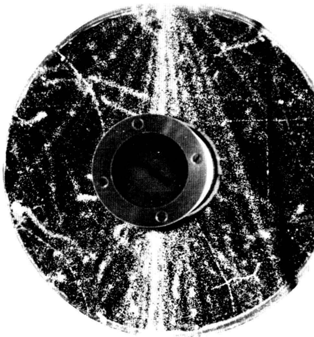
Plate 15. An electron shower, originating in a 2.5 cm. lead plate placed immediately over the cloud chamber.
