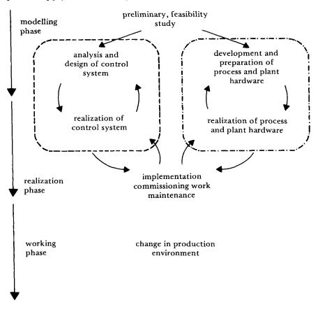
Figure 1.1 Development cycle of a control system:
