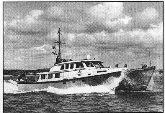
Photo 1.3 (a) The biggest fibreglass ships, the 470 ton minehunter, H.M.S. Sandown , built by Vosper Thornycroft, Southampton, England (Photo: Vosper Thornycroft Ltd). (b) The first large motor yacht, Bebe Grand , 55 ft (17 m), built by Halmatic Ltd in 1955 and still in service. Even after 30 years there were no blisters. To make a yacht of this size in those days needed much courage and faith at a time when most builders were making only dinghies – and people said even they had more faith than sense (Photo: Scott Bader Ltd).
