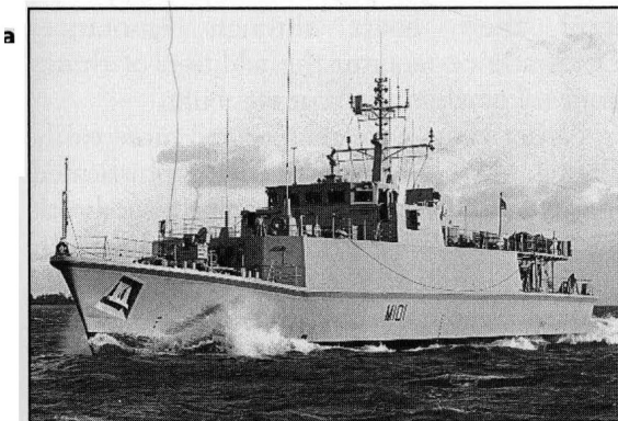
Photo 1.3 (a) The biggest fibreglass ships, the 470 ton minehunter, H.M.S. Sandown , built by Vosper Thornycroft, Southampton, England (Photo: Vosper Thornycroft Ltd). (b) The first large motor yacht, Bebe Grand , 55 ft (17 m), built by Halmatic Ltd in 1955 and still in service. Even after 30 years there were no blisters. To make a yacht of this size in those days needed much courage and faith at a time when most builders were making only dinghies – and people said even they had more faith than sense (Photo: Scott Bader Ltd).
