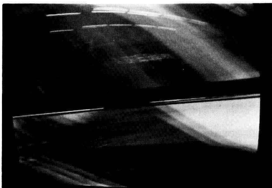
Figure 1-6 Sync pulses are used to lock the picture in the receiver. A loss of sync will often produce a picture such as this.
