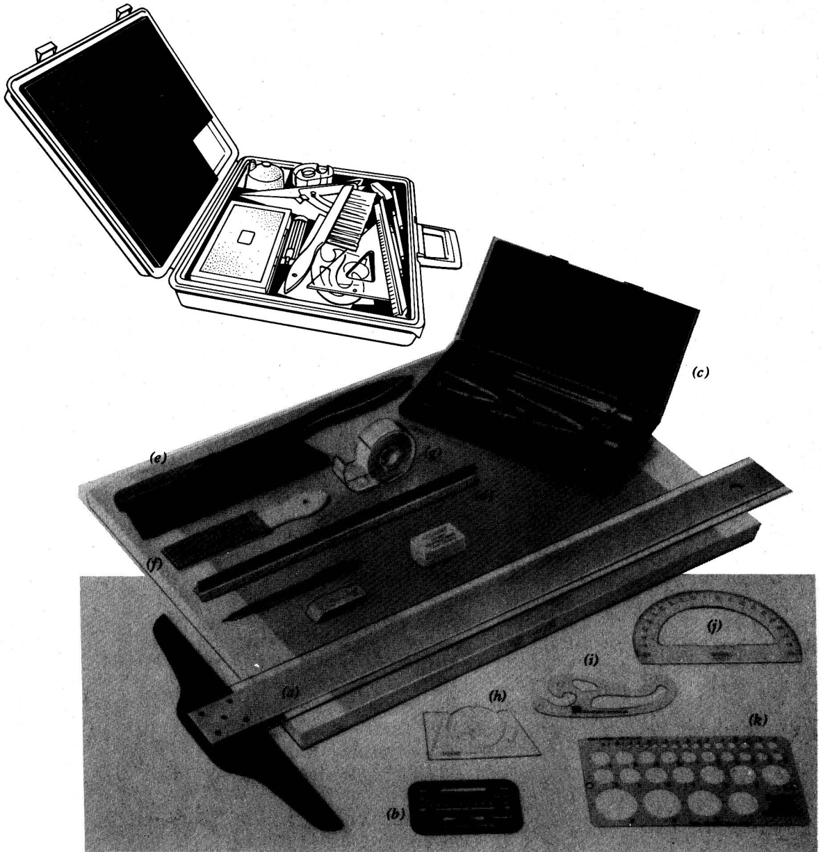
Figure 1-2 Drafting attache Case. (Courtesy of The Uteley Co., Inc.) (a) T-square; (b) erasing shield; (c) instrument case; (d) triangular scale; (e) dust brush; (f) sandpaper block; (g) drafting tape; (h) Ames Lettering Guide; (i) French curve; (j) protractor; (k) circle template.
