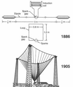
Heinrich Hertz's end-loaded half-wave dipole transmitting antenna and resonant half-wave receiving loop operating at  $\lambda=8$  m in 1886. The induction coil produced sparks at the gap in the dipole, resulting in sparks at the gap in the loop at a distance of several meters in Hertz's laboratory at Karlsruhe, Germany. This was the first radio link and the dipole and loop the first radio antennas.
