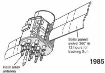
Helix antenna array on one of 24 Global Position Satellites (GPS) in Medium Earth Orbit (MEO) at 20,000 km. Operating at  $\lambda \cong 20$  cm, these satellites provide you on or above the earth with your position (latitude, longitude and elevation) to an accuracy of better than 1 meter.
