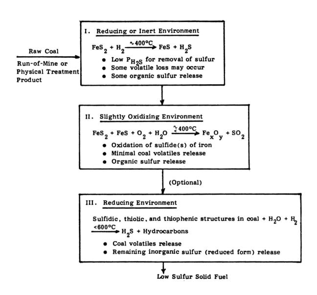
Figure 1-1. Westinghouse Coal Pyrolysis Process Concept
