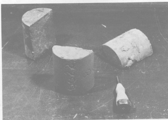
Fig. 6. Soil-cement specimens saved from tail end of moisture-density test procedure. Rate of hardening of the soil-cement mixture is investigated from day to day with a dull-pointed instrument.
